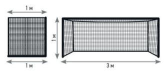
Water polo presents a unique application problem. The acids and chlorine found in pools can eat up an average net in no time. That is why our specially treated water polo netting uses HTPP that is specifically manufactured to resist acid and chlorine for a longer goal life.
